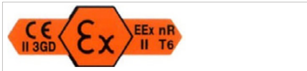
Figure 19: Example of a plate attached to a gas detector
